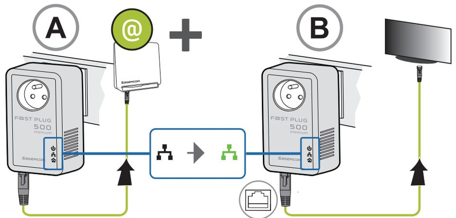
Recommended use of a multiple plug adapter
